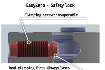
This safety lock has especially been developed for the EasyZero zero point system. It secures clamping devices and workpieces mechanically and insuperably on the machine table. An opening of the safety lock due to overload is impossible - the clamping screw or clamping stud would have to be smashed for this.
