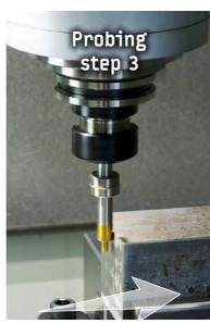
3. When reaching the final position, the edge finder body passes along the edge. Now, the position corresponds to the radius of the
