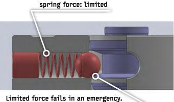
Spring force, however, is limited and fails at high machining forces and in an emergency. Dirt can also reduce the spring force and allow risky opening. This usually provokes a crash which can lead to damage to the workpiece, tool or machine and can even cause injury to the machine operator.
